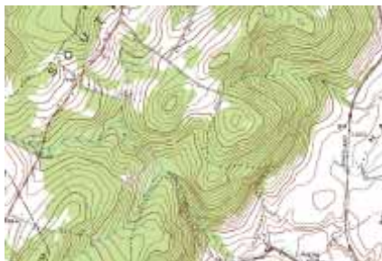
Figure 3. Example of a contour map. The lines identify areas of varying elevation.
